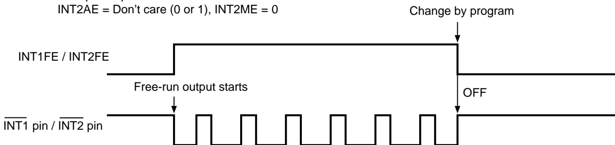
Figure 27 Output Timing of User-set Frequency
